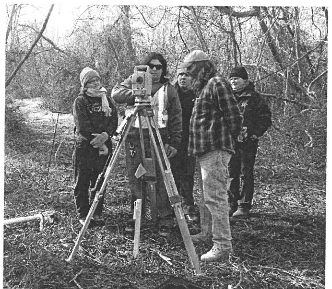
Total station transit used by Maryland State Highway Administration Survey Team and Lost Towns Project archaeologists at Curtis Creek Site.
