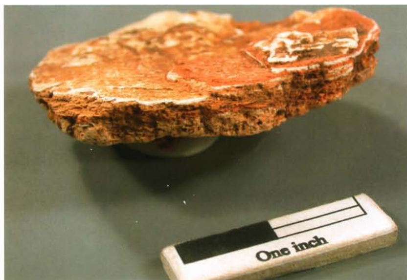
Figure 19 Repeated application of a clay wash on the muffle interior produced a laminar structure called “lute.” (Photo, David Gadsby.)
