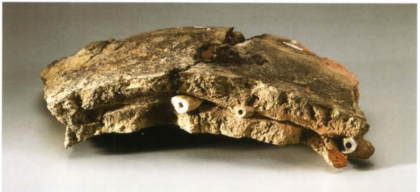
Figure 16 A fragment of the muffle showing the utilization of broken pipe stems as a bond between coils during construction. (Photo, Gavin Ashworth.)
